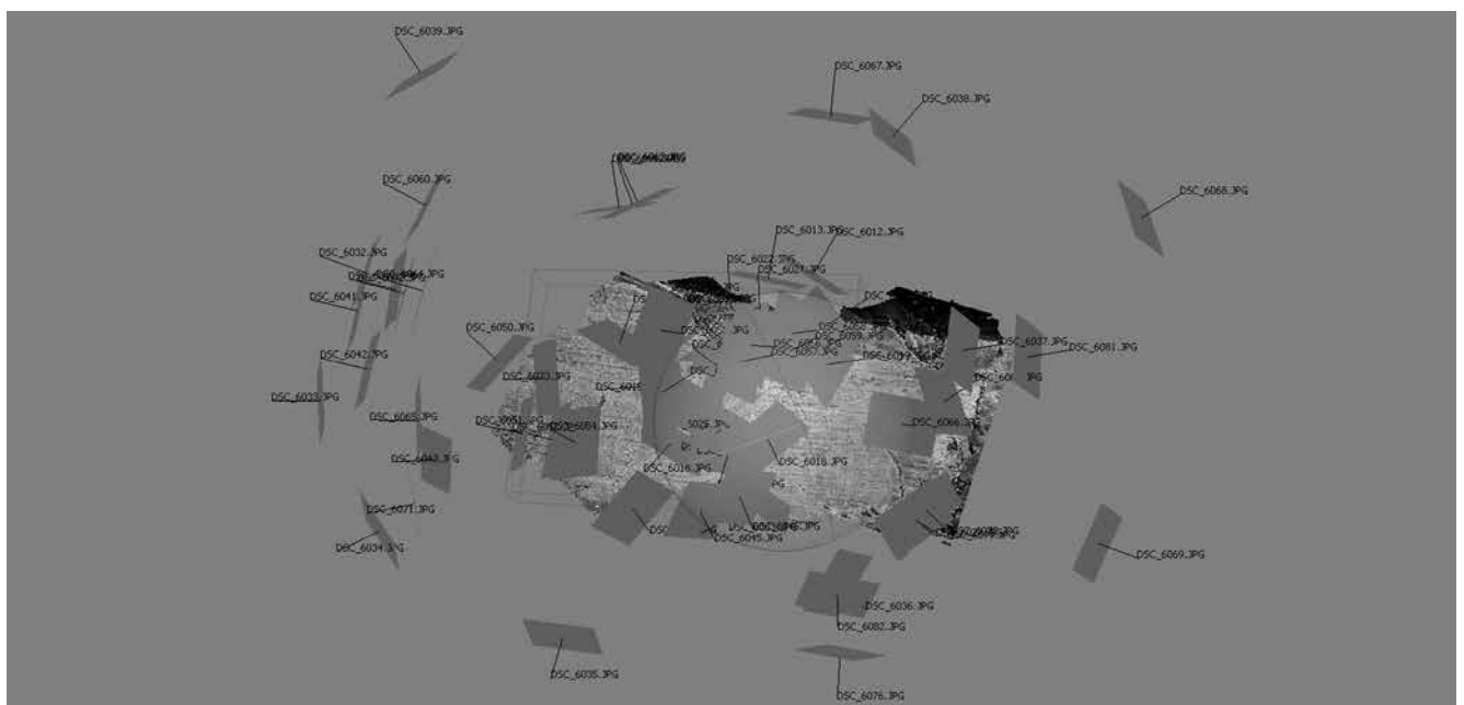
Fig. 3 - A view of the reconstruction of some squares with the positions from where the shoots were taken.
